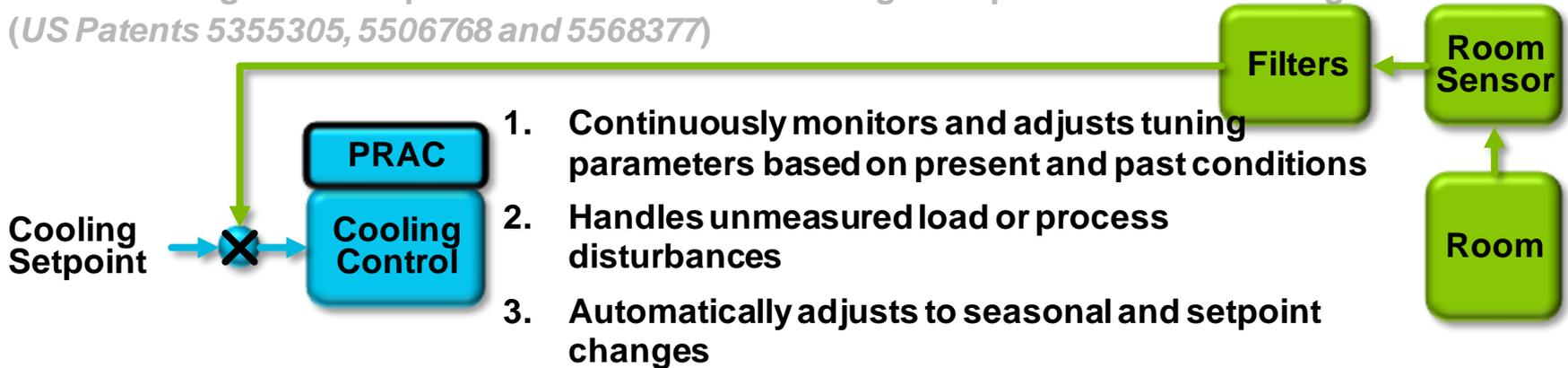
1. Continuously monitors and adjusts tuning parameters based on present and past conditions
