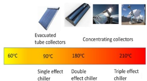
Solar collectors and absorption chiller mapping based on temperature
