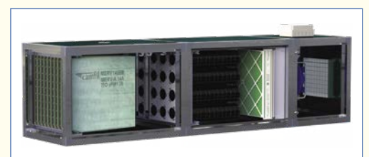
Example of large-scale modular air cleaner configuration showing particulate bag-style pre-filter, molecular canister-style housing filled with pelletised media, final safety particulate panel filters, and fan system.
