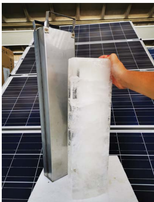
Solar Cooling Engineering UG in Germany sees ice being used as a "cooling battery".
