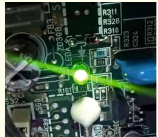
Figure 4: A printed circuit board monitor light flashes to indicate status and health of a CPU, but this may turn off when the unit is in passive standby mode. Source: Dennis Kenworthy
