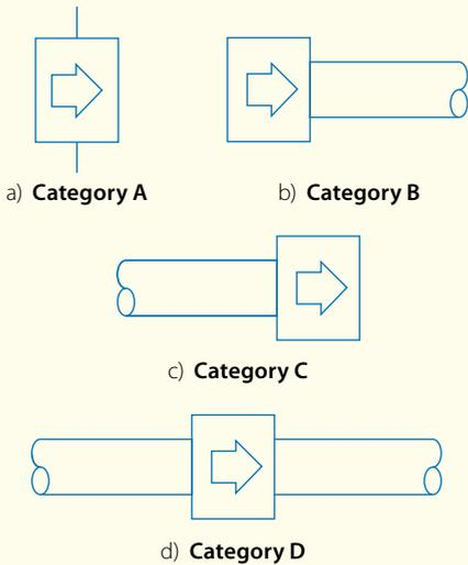
Figure 1: Fan test configuration categories.
