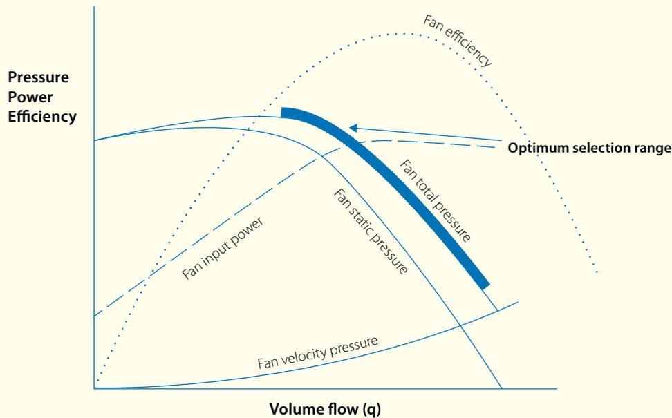
Figure 3: Fan performance curves showing recommended selection range.
