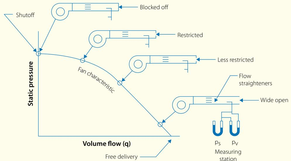
Figure 2: The creation of a fan performance characteristic.
