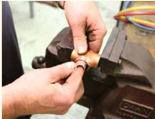
Fig 3: Cleaning tubing ends and fitting sockets.
