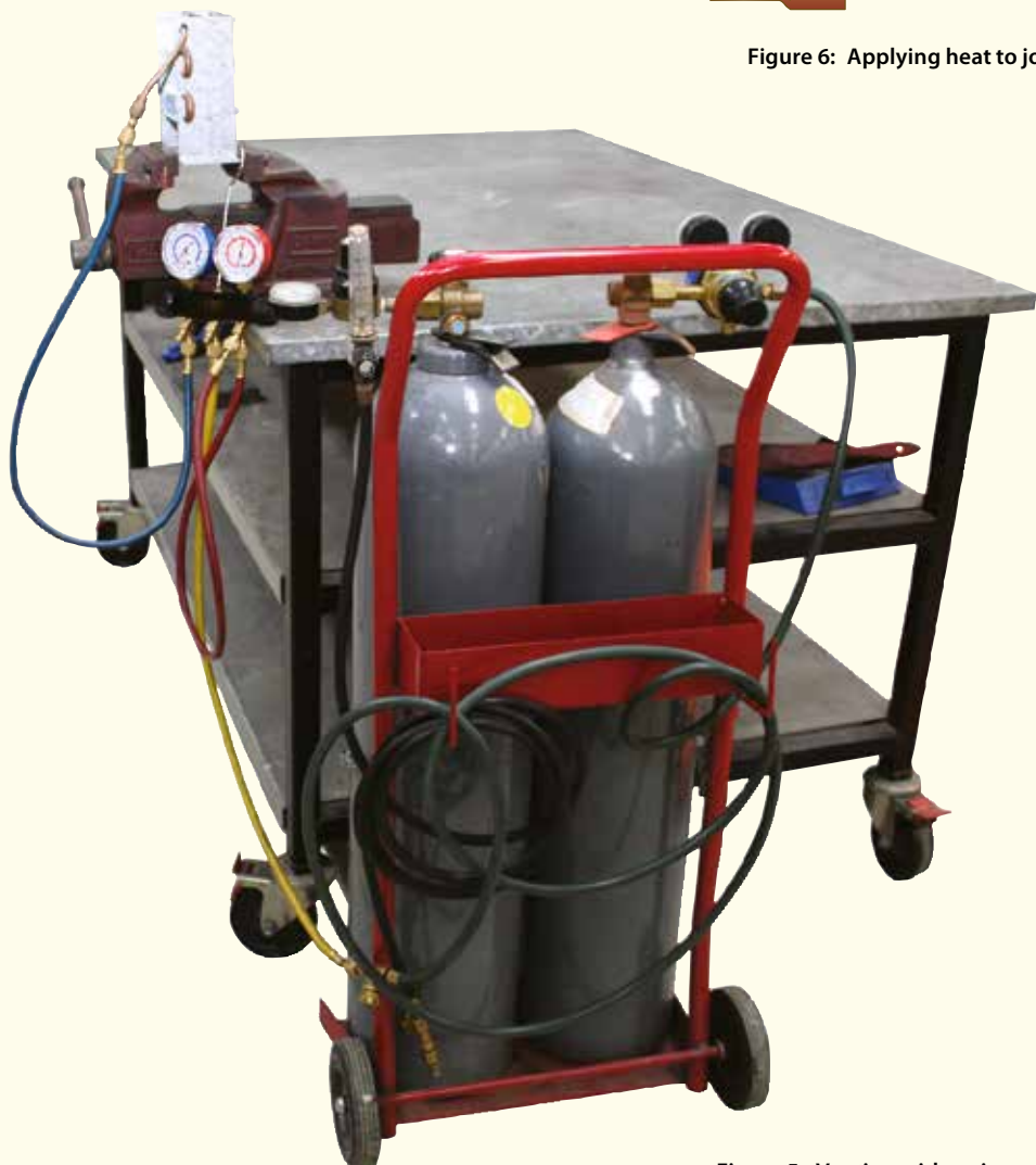
Figure 5: Venting with an inert gas.
