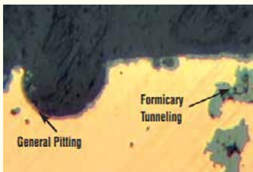
Formicary corrosion tunneling.
