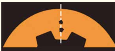
Cross-section showing portion of corrosion (leak).
