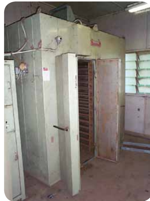
Drying cabinets containing heater banks with asbestos lining and textile wrapped electrical wiring.
