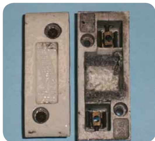
Ceramic fuse holder with a textile spark/flare arrester.
