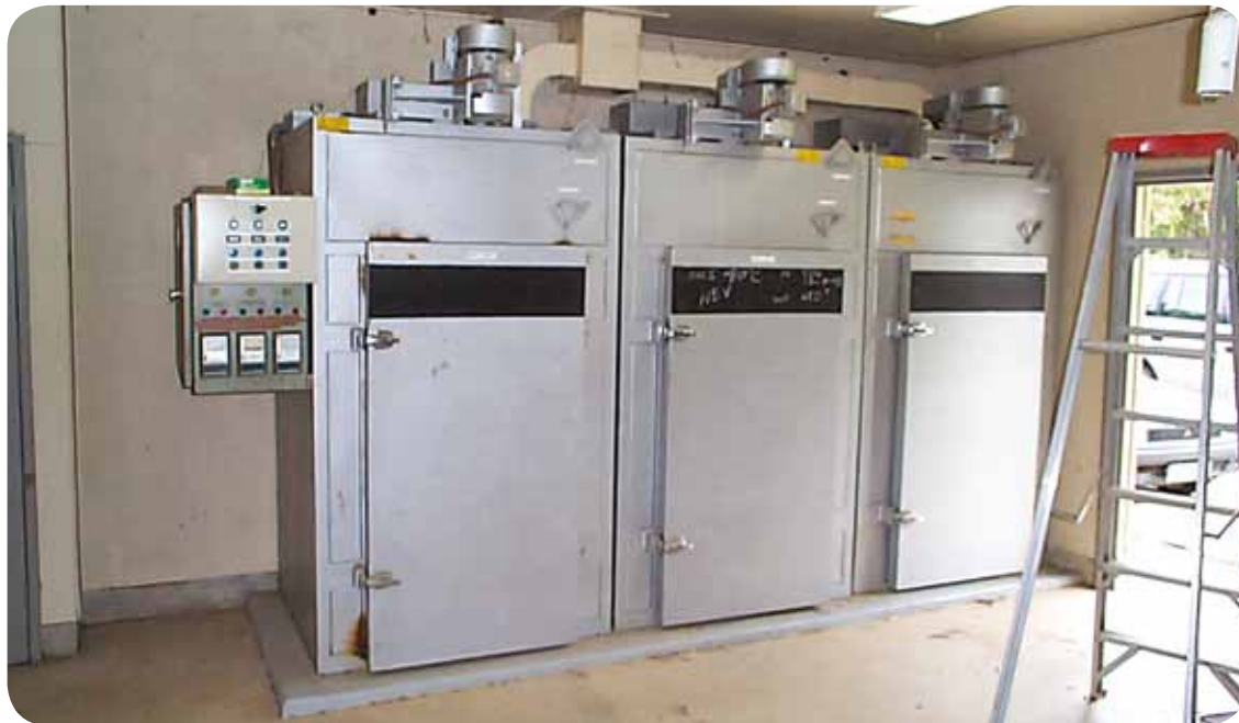
Drying cabinets containing heater banks with asbestos lining and textile wrapped electrical wiring.
