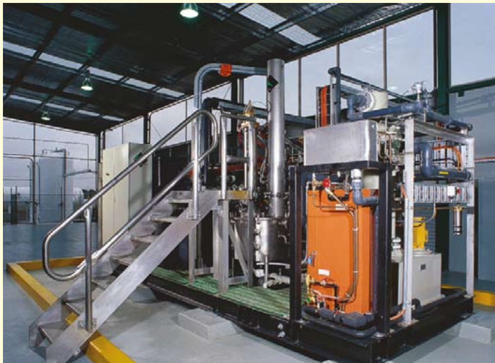
Plasma arc machine – used by RRA to destroy refrigerants at the end of their useful life
