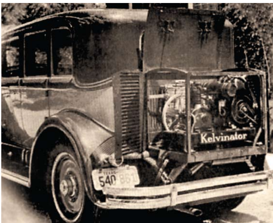
Fig 1 – The first car air conditioned by C&C Kelvinator Co. for John Hamman Jr. of Houston, Texas in 1930.
