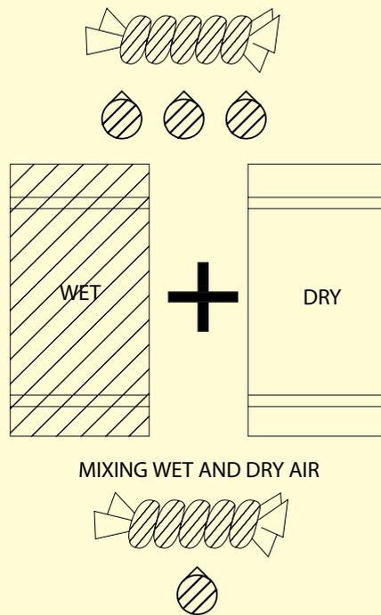
dry towel will not prevent some of the water from dropping out when the two are compressed. Because of this, some pumps are designed to run with both high internal temperatures (to reduce moisture condensation in the oil) and a gas ballast.
