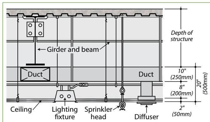
Figure 2: Typical Ceiling Plenum Space
