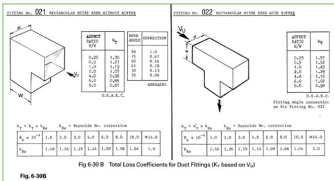
Figure 3: DA03 Fitting 021 and Fitting 022 Rectangular bends.
