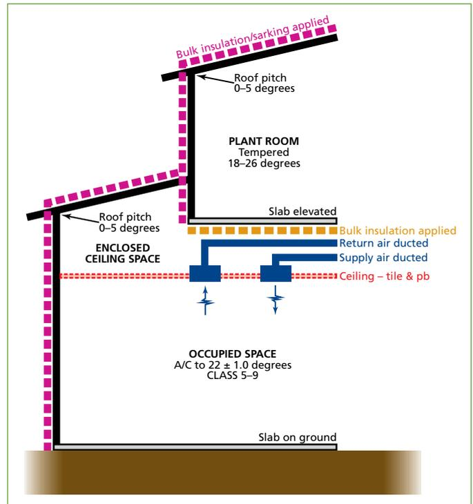
Figure 1: Building envelope diagram
