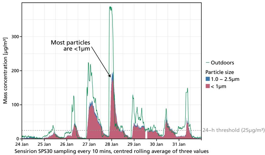
Figure 3: Smoke infiltration in an extremely airtight building
