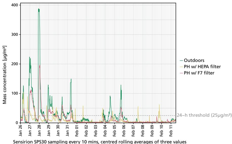
Figure 4: Two identical airtight homes with mechanical ventilation, one with a standard F7 filter and the other with a HEPA filter
