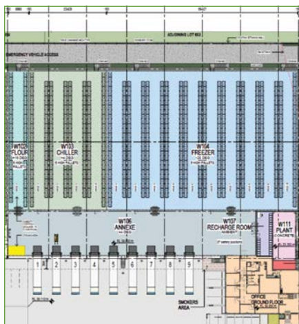
Figure 1. Perth facility in plan view
