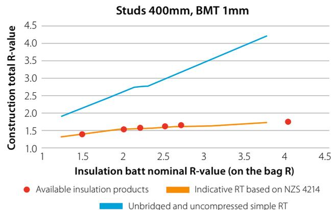
Figure 3: Metal framed wall total R-value, calculated according to NZS 4214 for a range of insulation thicknesses and compared with the unbridged R-values. Note the “kick” in the unbridged graph occurs at the point where the thickness of the insulation fully fills the gap in the frame so that there is no air layer inside the insulation.
