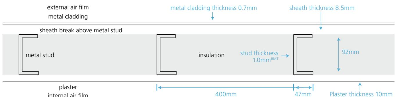
Figure 1: Plan view through metal-framed wall.
