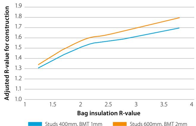
Figure 4: Metal framed wall total R-value, calculated according to NZS 4214 for a range of insulation thicknesses and two different frame geometries.
