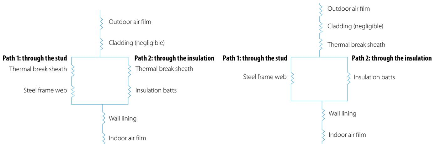
Figure 2: Different concepts of heat-flow pathways through the metal-framed wall. The diagram on the left was used for the calculation (i.e., isotherms for the bridged layers were drawn outside the thermal break sheath, even though it is a homogeneous material).
