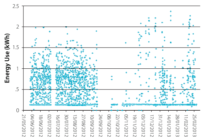
Figure 3.1: Daily operation of an air conditioner over three seasons in Adelaide houses.
