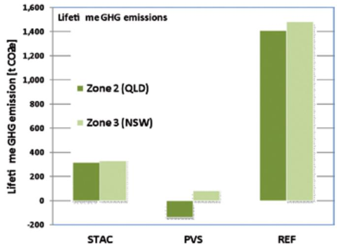
Figure 5. Lifetime greenhouse gas emissions of all systems
