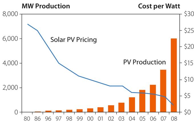
Figure 1. Global PV production and PV panel price from 1980 – 2008 [20].
