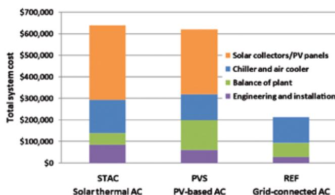
Figure 3. Breakdown of system equipment and installation costs.
