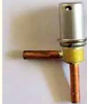
Figure 1. Electronic stepper valves have very little moving parts and a simple construction. They can bi-flow easily and work with very little port-pressure as long they have subcooled liquid. These have been a major factor in efficiency increases to domestic and commercial air-conditioning systems. They allow better COP/EER, through effecting good flow capacity and lower superheats at varying ambient conditions.
