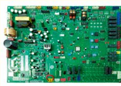
Figure 3. Electronic expansion valve control panel for an air conditioning unit.
